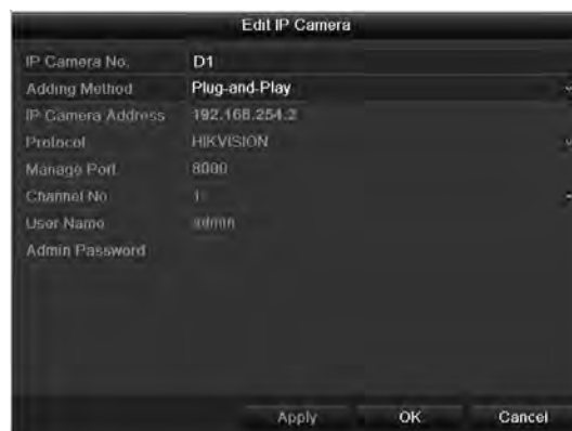
Figure 2. 27 Edit IP Camera Interface - Plug-and-Play
