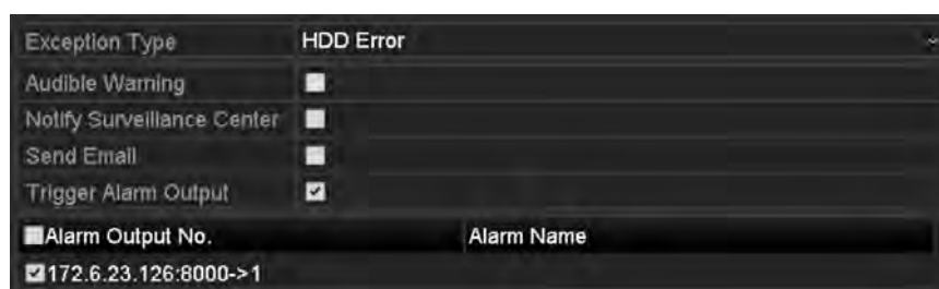
Figure 10. 22 Configure HDD Error Alarm
