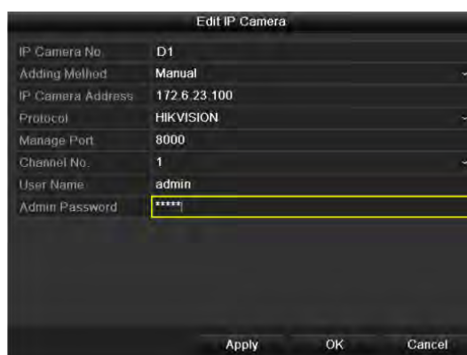
Figure 2. 28 Edit IP Camera Interface - Manual
