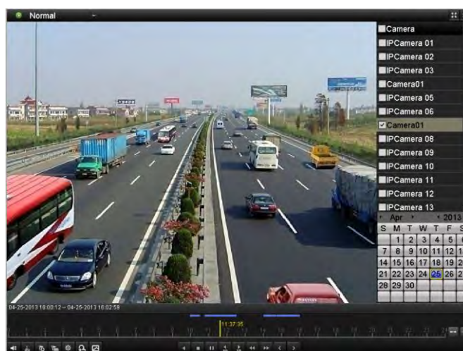
Figure 6.6 Interface of Playback by Time
