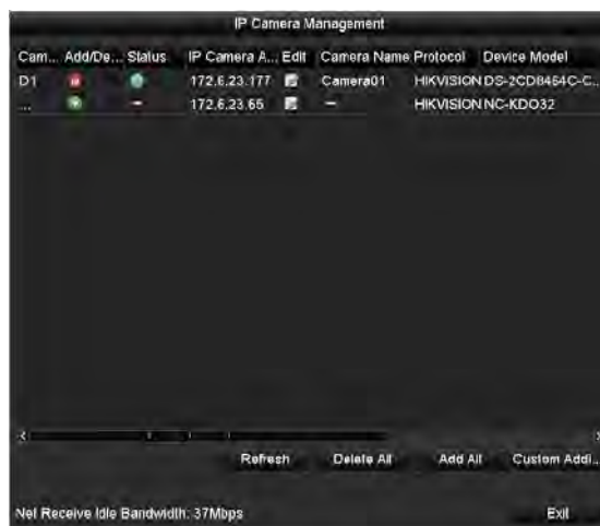
Figure 2. 13 Manual Adding IP Camera Interface
