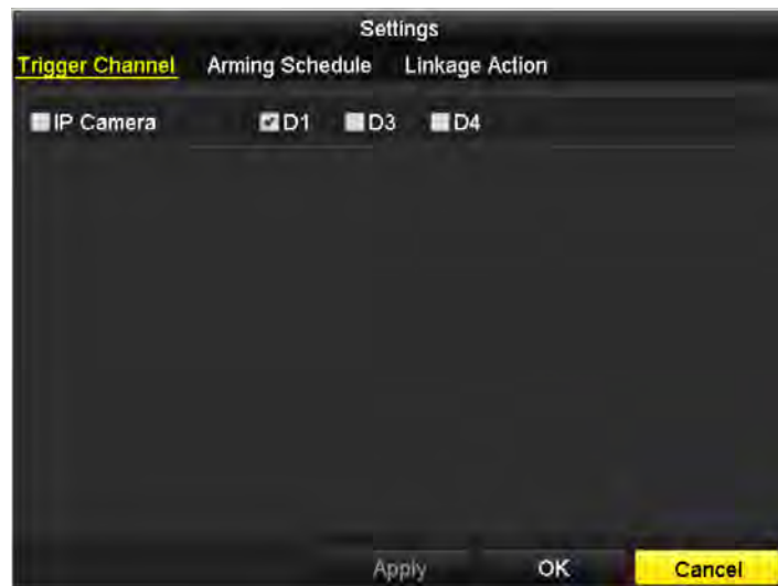
Figure 5. 14 Motion Detection Setting
