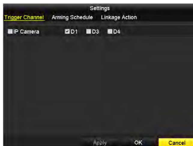
Figure 8.2 Set Trigger Camera of Motion Detection
