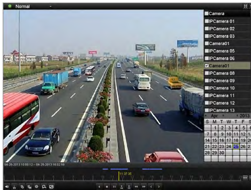
Figure 6.13 Interface of Playback by Time
