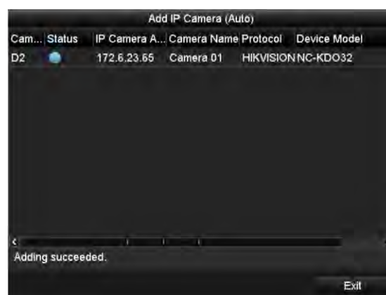
Figure 2.12 Auto Adding IP Camera Interface
