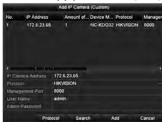
Figure 2. 14 Custom Adding IP Camera Interface
