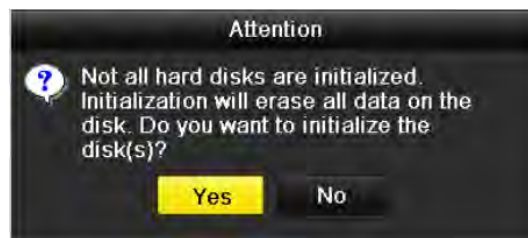
Figure 10.1 Message Box of Uninitialized HDD
