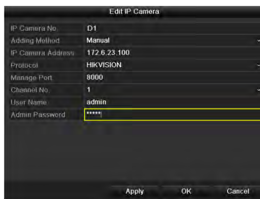
Figure 2. 25 Edit IP Camera Interface - Manual
