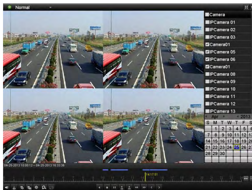
Figure 6.27 4-ch Synchronous Playback Interface
