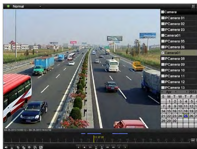
Figure 7.21 Interface of Playback by Time
