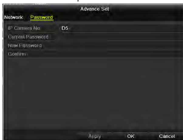
Figure 2. 20 Password Configuration of the Camera
