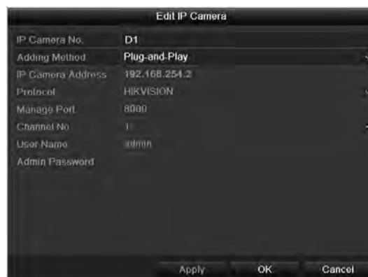
Figure 2. 24 Edit IP Camera Interface - Plug-and-Play
