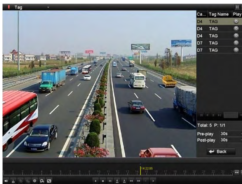
Figure 6.16 Interface of Playback by Tag
