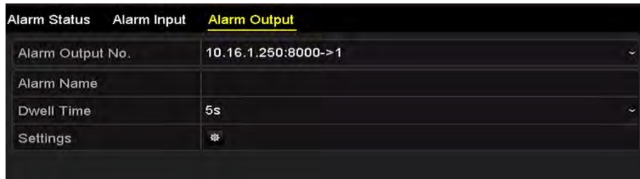
Figure 8-21 Alarm Output Settings Interface
