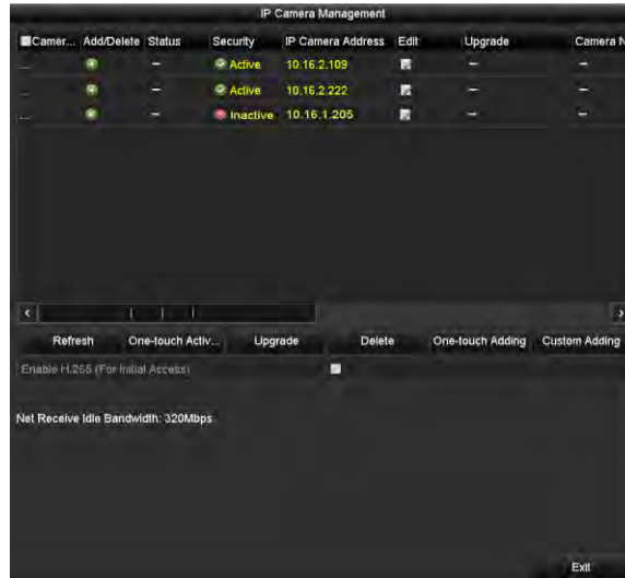
Figure 2-38 IP Camera Management Interface
