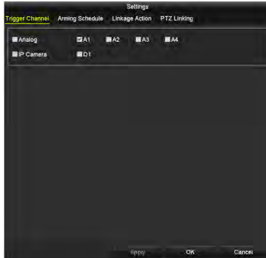
Figure 5-22 Set Triggered Camera of VCA Alarm
