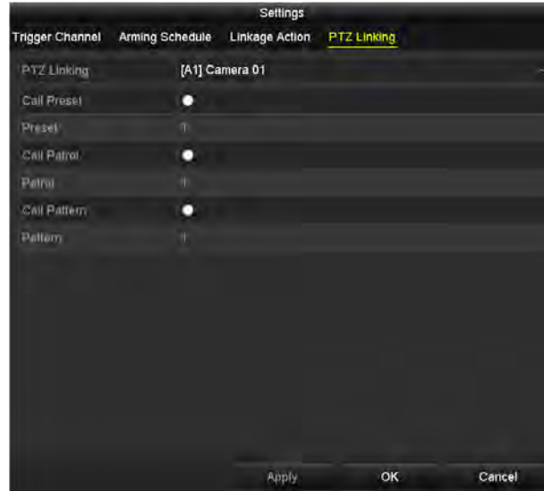
Figure 8-9 Set PTZ Linking of Alarm Input
