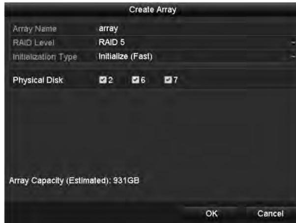
Figure 13-8 Create Array Interface
