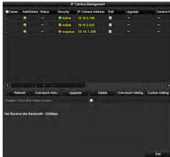
Figure 2-38 IP Camera Management Interface
