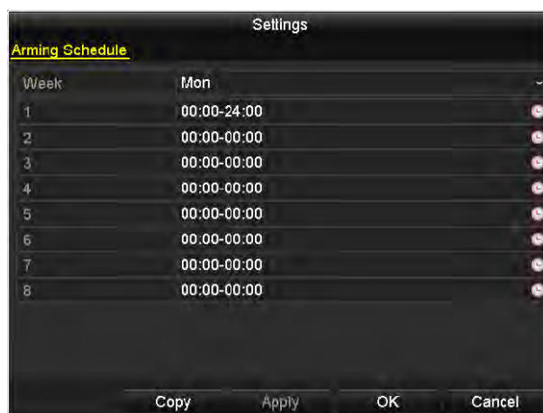
Figure 8-22 Set Arming Schedule of Alarm Output
