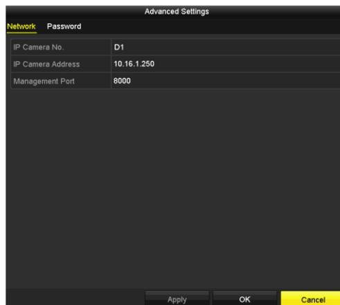
Figure 2-46 Network Configuration of the Camera
