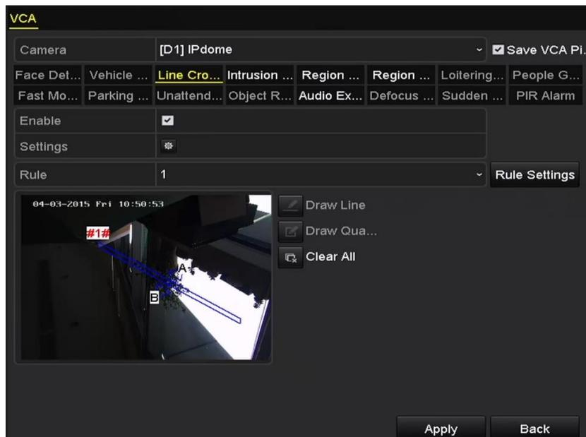
Figure 10-7 Draw Line for Line Crossing Detection
