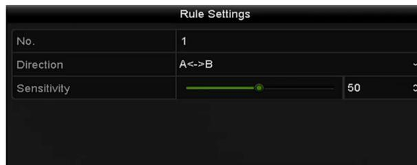
Figure 10-6 Set Line Crossing Detection Rules
