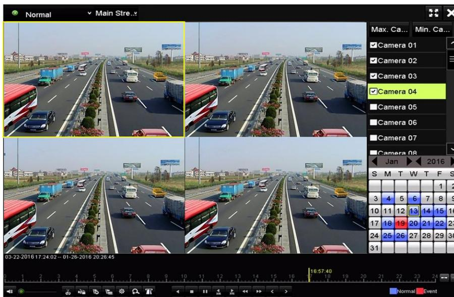
Figure 6-26 4-ch Synchronous Playback Interface
